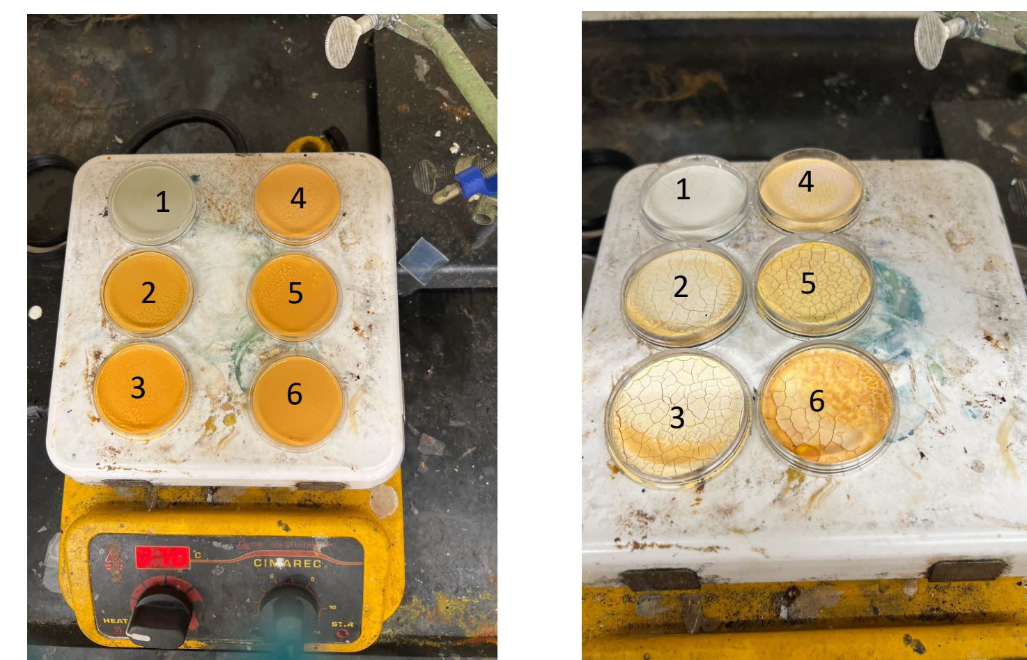
Figure 4. Samples before and after 24 hours on hot plate
